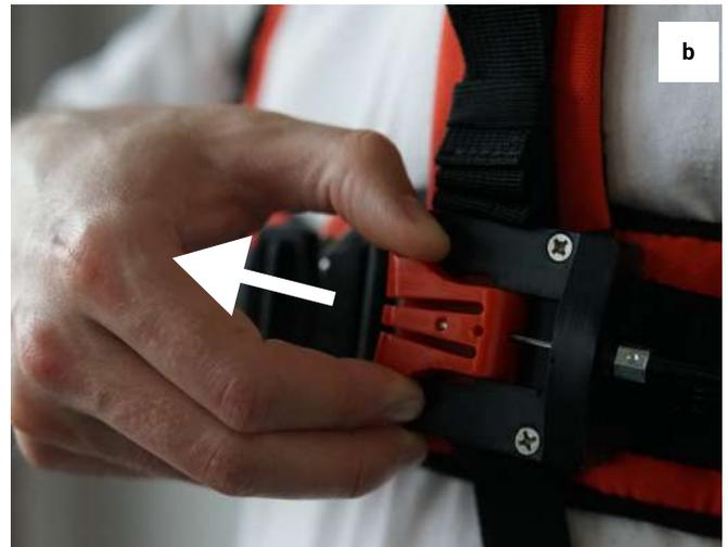
Figure 4: Turn OFF the exoskeleton mechanism by setting the ON/OFF button to OFF.
