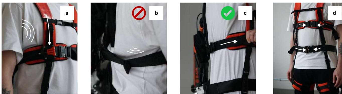
Figure 14: Straps friction under the arms.
