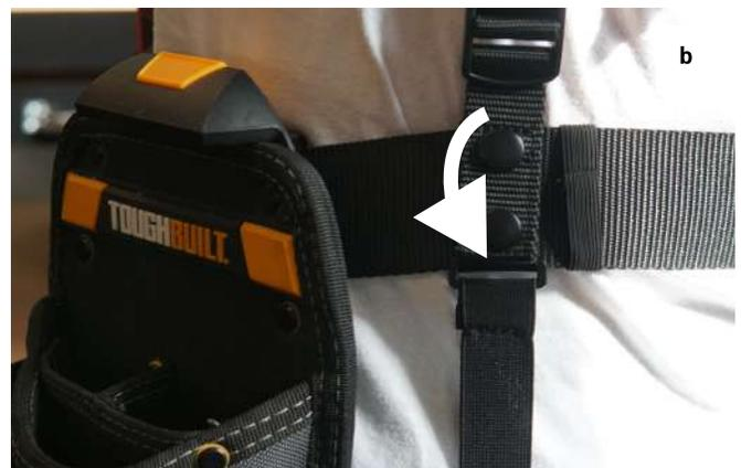
Figure 5: Fitting the personal tool bag to the Biolift exoskeleton.
