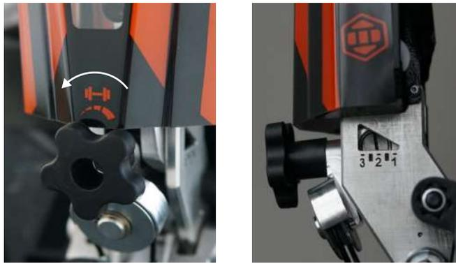
Figure 12: Support adjustment.
